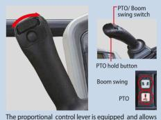
you to control boom swing operation and the attachment easily.
