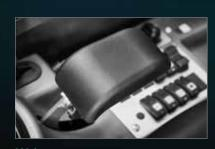
Wrist rests Wrist rests on the each control lever box ensure fatigue-free operation.
