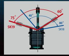
Wide boom swing angle The boom swing angle has been 12% wider than that of SK18.
