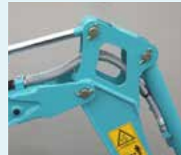
Bucket cylinder hose inside the arm
