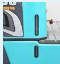
Fuel tank gauge that shows the fuel level at a glance.
