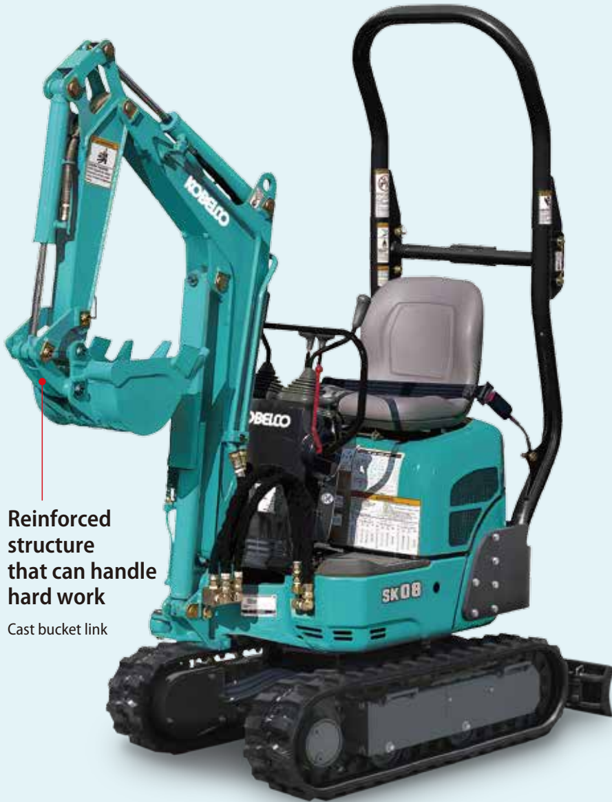
Bucket cylinder hose inside the arm
