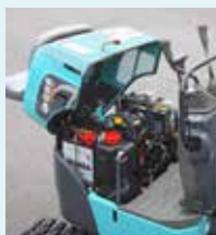
Fully opening hood for large access space.
