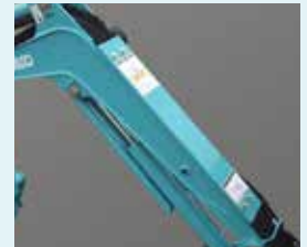
Hose protection cover on back of boom
